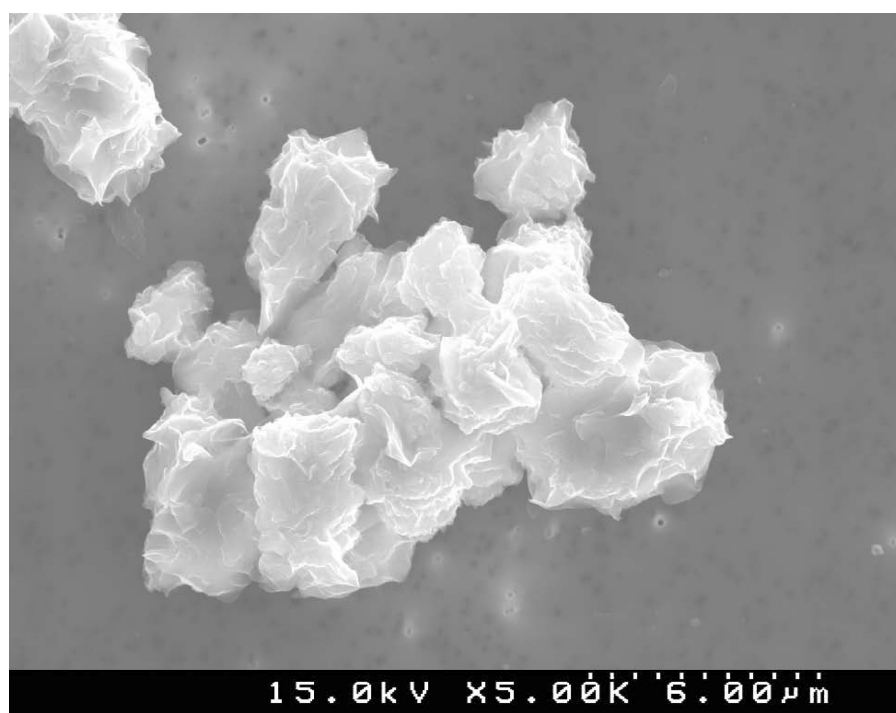
FIG. 4. Quartz isolate before instillation (5000 \times ).
